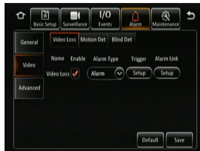
Video Loss Alarm Figure 99
